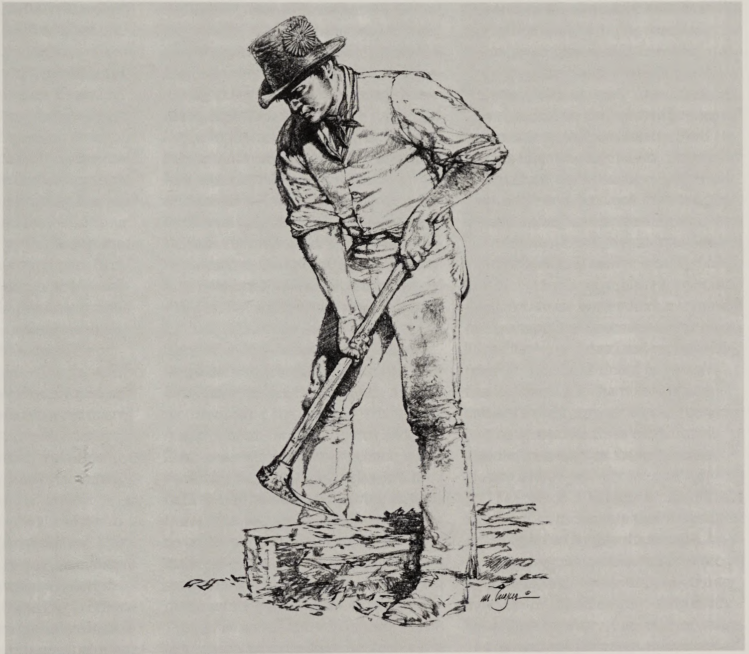
Sgt. Patrick Gass, in this drawing squaring a log with an adze, was the Corps of Discovery's head carpenter.
